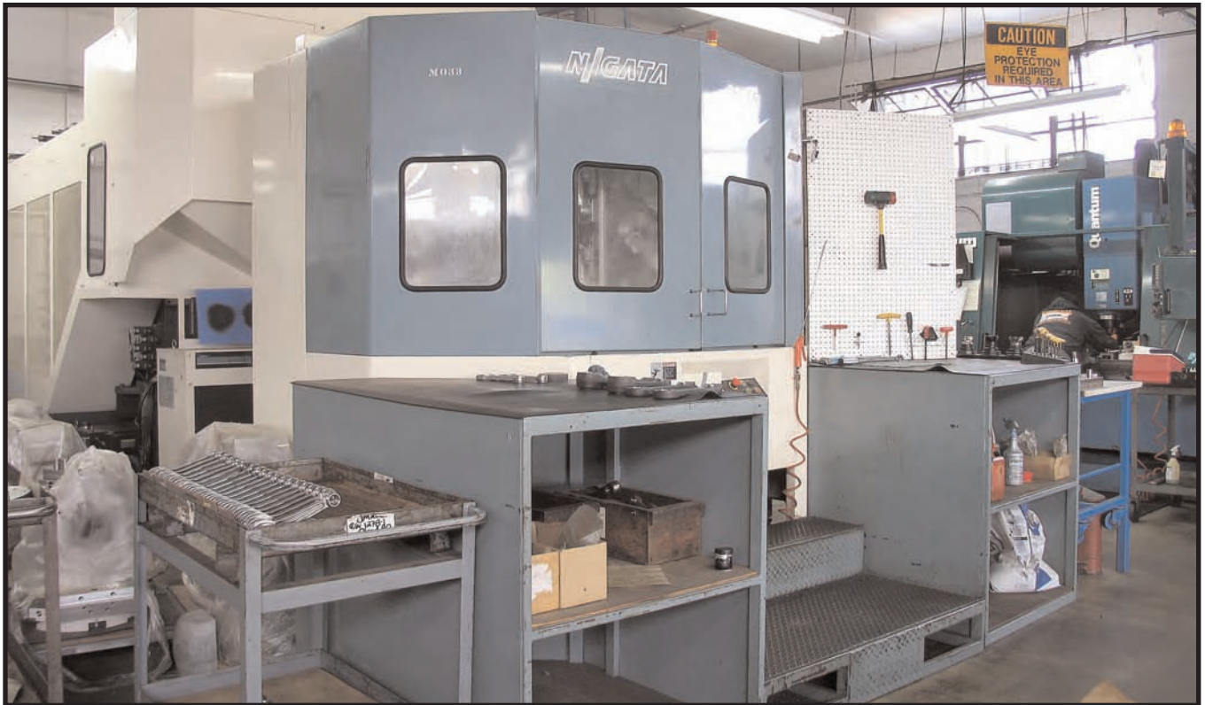
Niigata 50 Taper Horizontal Mill – Full 4th Axis - Model No. SPN63
