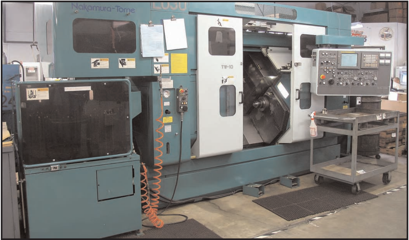
Nakamura Twin Spindle CNC Lathe TW-10 With Milling and Gantry Parts Loader
