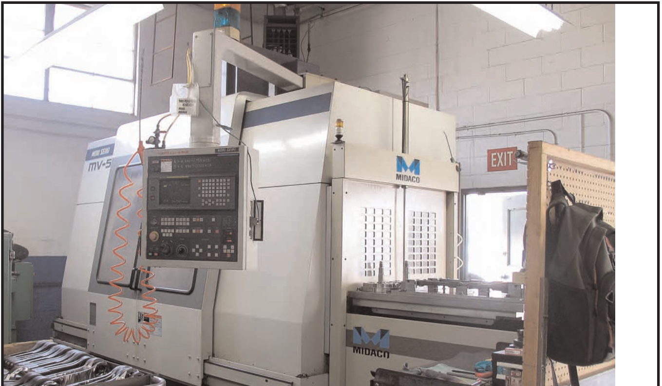
Mori Seiki 50 Taper Vertical Mill 6,000rpm Spindle
